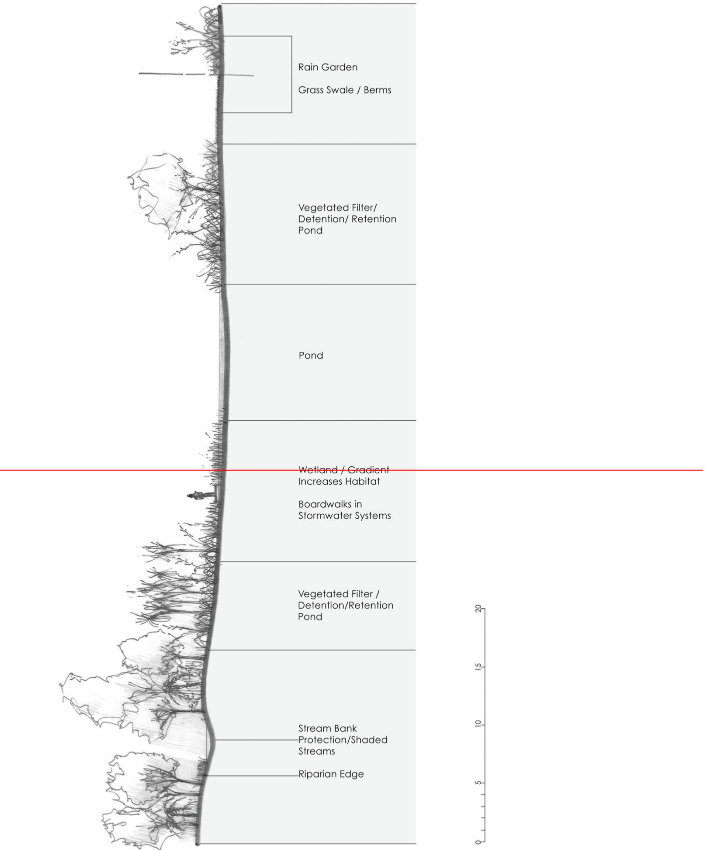
Figure 4. Typical cross-section of Stormwater Management demonstrating the structure and composition of a range of stormwater devices.
